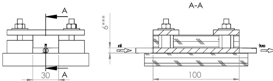
**Fig.3. Dimensions of the experimental cell (from [21])**
