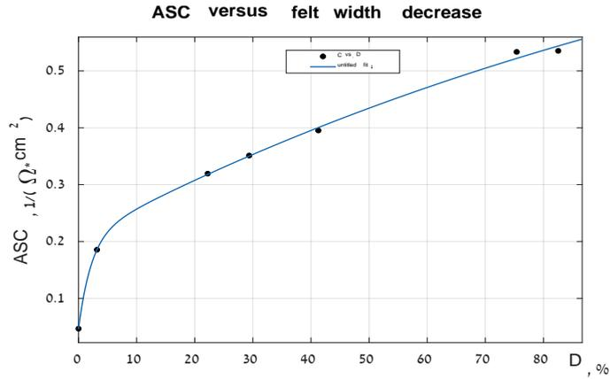
**Fig.4.** ASC of a dry CF versus relative felt decrease.
