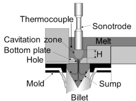
Figure 7. A representation of unit for hot-top UST casting with controlled melt flow.
