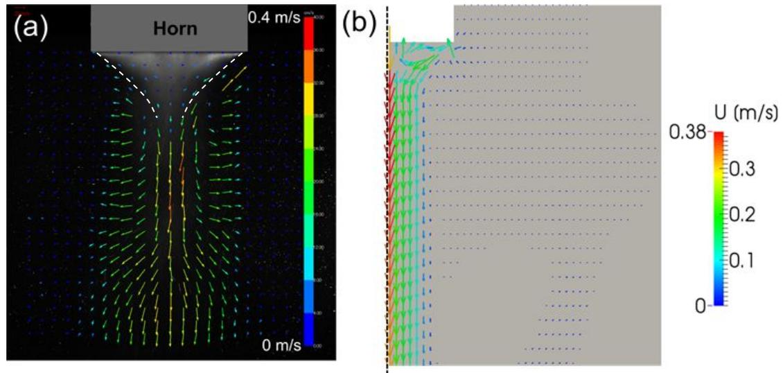
Figure 5. Typical vectors of acoustic streaming velocity obtained experimentally (a) and numerically (b).
