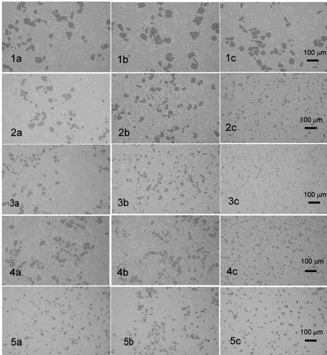
Figure 4. Microstructure images of samples taken at the center (a), half-radius (b) and surface (c) of a 178-mm billet produced by different casting methods : the conventional casting (1), launder UST casting (2), hot-top UST (3,4) casting, novel hot-top UST casting with controlled melt flow (5).
