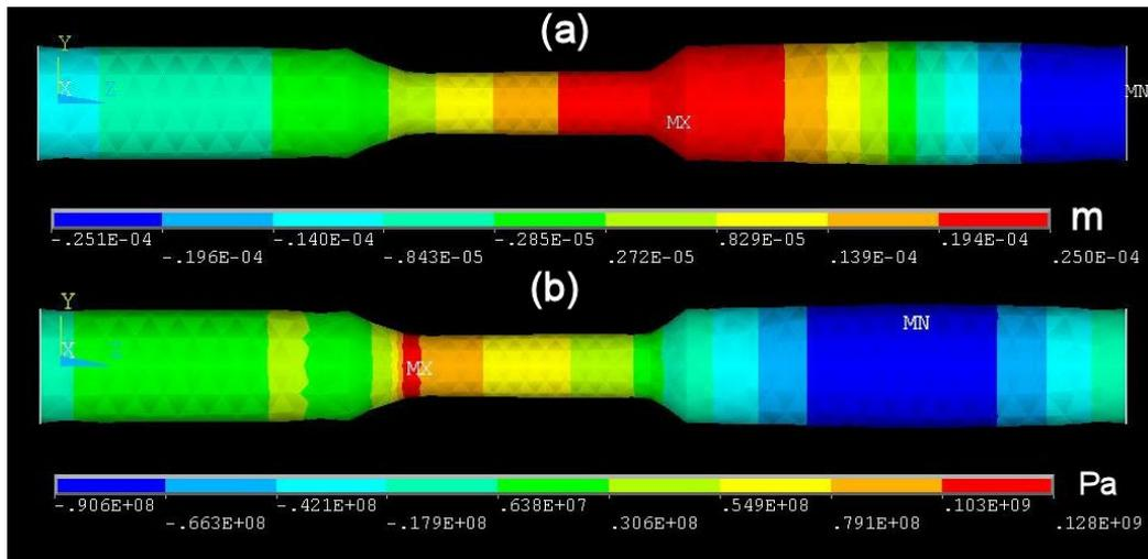
Figure 1. Lengthwise distributions of displacement (a) and internal stress (b) amplitudes.
