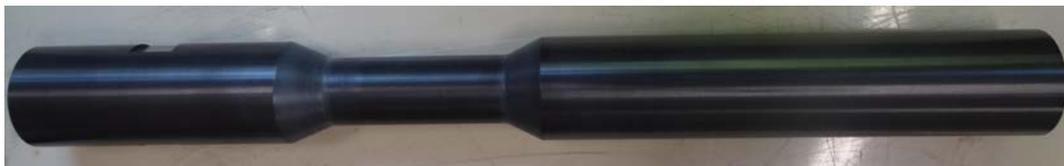
Figure 2. Appearance of barbell ceramic sonotrode
