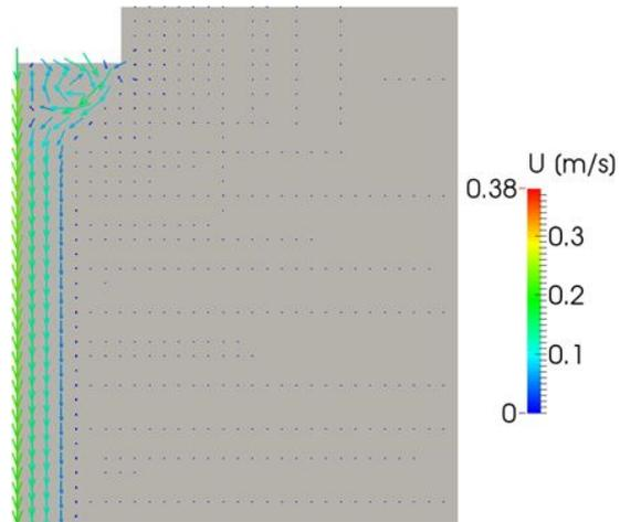
Figure 6. Predicted vectors of acoustic streaming in molten aluminum at  $A=40 \mu\text{m}$
