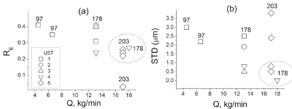
Figure 8. Dependence of  $R_E$  and  $STD$  index on metal flow rate: 1: launder UST, 2,3: hot-top UST, 4,5 : improved hot-top UST.
