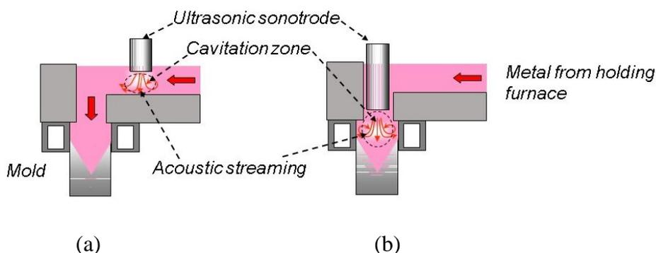
Figure 3. A representation of (a) launder UST and (b) hot-top UST casting.
