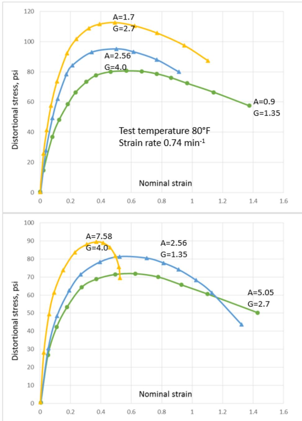
Fig. 6. Comparison of the effect of the sample size upon the mechanical properties of the particulate reinforced rubber-like material.
