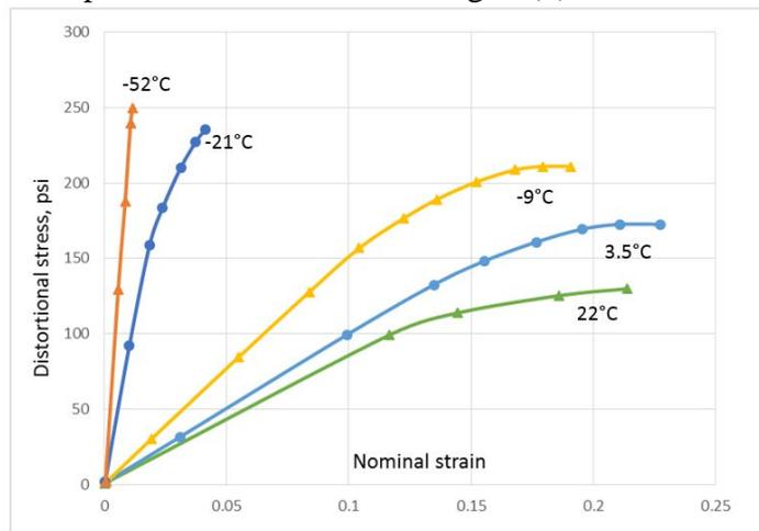
Fig. 5. Temperature effect particulate reinforced composites.
