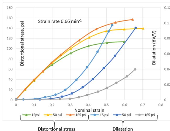
Fig. 1. Nonlinear stress-strain behavior of particulate reinforced rubber-like material for different superimposed hydrostatic pressures (15, 50, 165 psi ) during uniaxial tensile test.
