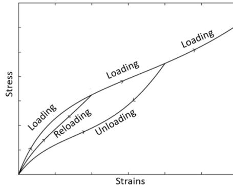
Fig. 4. Schematic loading-unloading-reloading curves in simple tension for the material which possesses Mullins effect.
