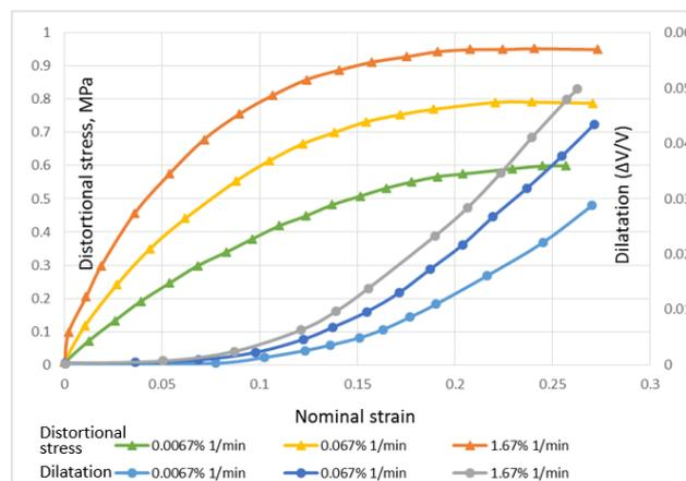
Fig. 2. Nonlinear stress-strain behavior of particulate reinforced rubber-like material for different strain rates (0.0067%, 0.067%, 1.67% min<sup>-1</sup>) during uniaxial tensile test.
