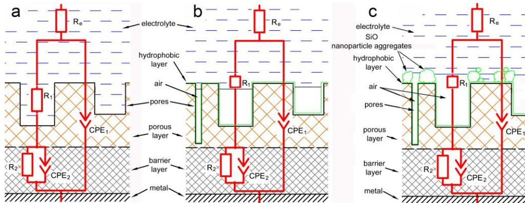
Fig. 6. Graphical representation of electrolyte/coating interface and equivalent electrical circuits used for fitting the experimental impedance data for aluminum alloy samples: a – PEO, b – PEO + MAF, and c – PEO + MAF +  $\text{SiO}_2$ .
