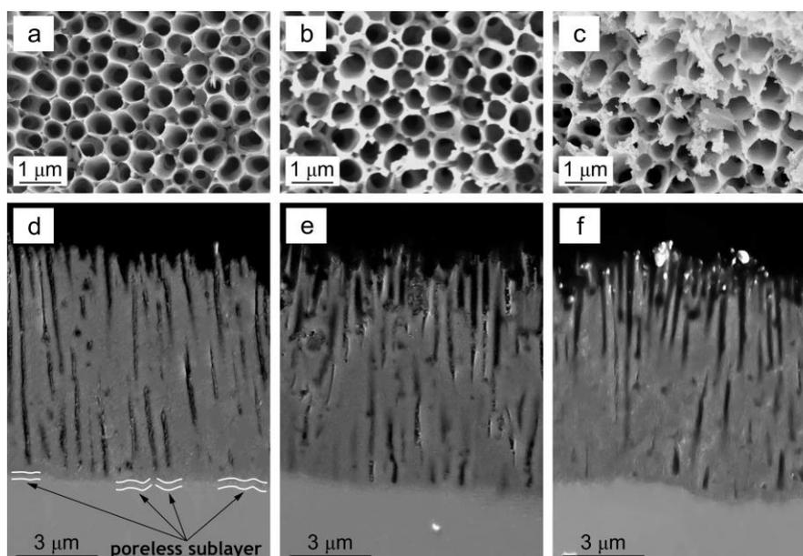
Fig. 1. SEM-images of the surface (a, b, c) and cross-sections (d, e, f) for coatings: PEO (a, d), PEO + MAF (b, e), and PEO + MAF + SiO<sub>2</sub> (c, f).
