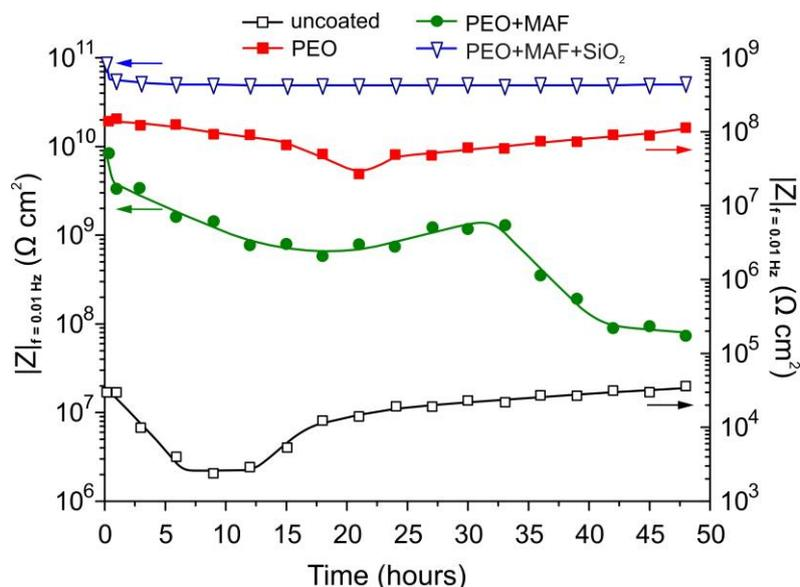
Fig. 7. The evolution of the impedance modulus values measured at 0.01 Hz with time during exposure of the samples to 3% NaCl solution for 48 h.
