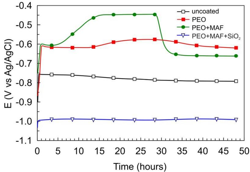
Fig. 3. OCP evolution during the exposure of the samples to 3 % NaCl for 48 h.
