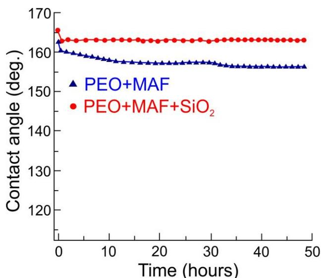
Fig. 2. The evolution of the contact angle with time after deposition of the drop of 3 % NaCl aqueous solution on samples.
