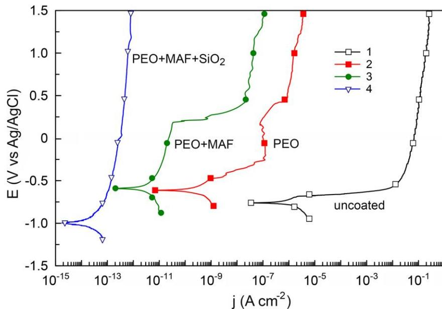
Fig.4. Polarization curves obtained in 3 % NaCl solution for the aluminum alloy samples with different surface layers: 2 – PEO, 3 – HP-coating formed by deposition of hydrophobic agent monolayer atop the PEO-coating (PEO + MAF), 4 – nanocomposite SHP-coating formed by aggregation of silica nanoparticles (PEO + MAF + SiO<sub>2</sub>). Curve 1 – for the uncoated sample provided for comparison.
