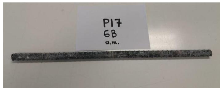
Fig. 9 – Smooth steel bar collected in one RC column used to tensile test.
