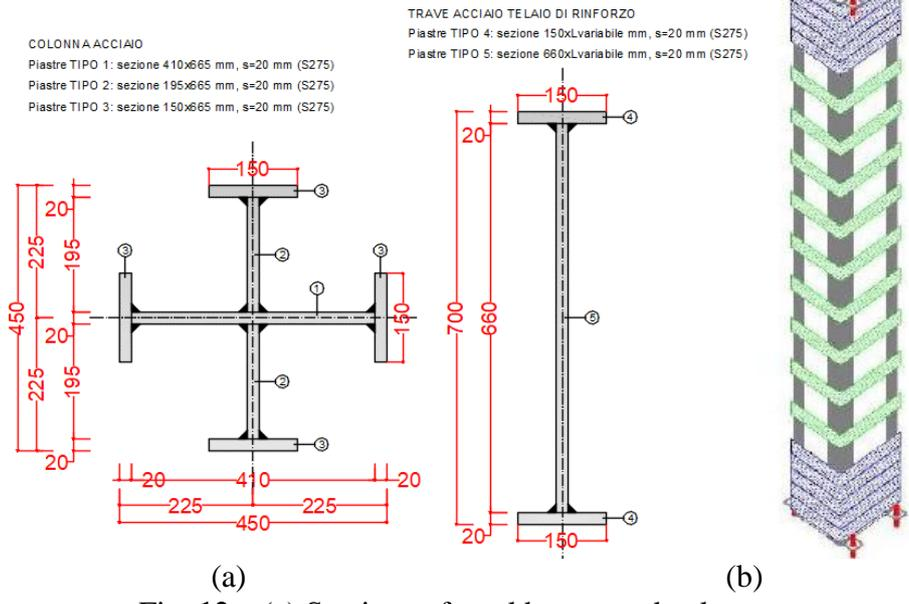
Fig. 12 – (a) Sections of steel beams and columns.
