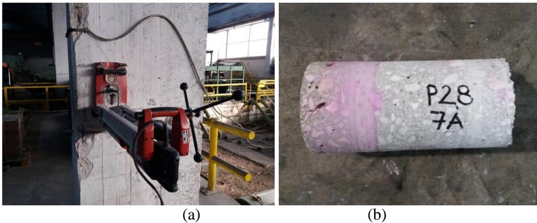
Fig. 8 – (a) Extraction of concrete sample and (b) element to test in laboratory.
