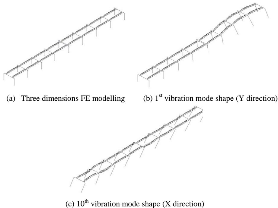
Fig. 10 – FE modelling and mode shapes of RC frames
