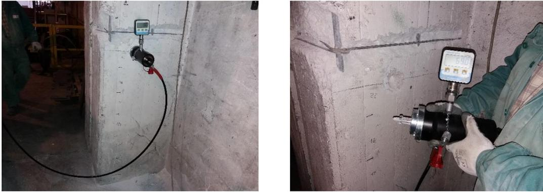
Fig. 7 - Pull-out tests on RC columns
