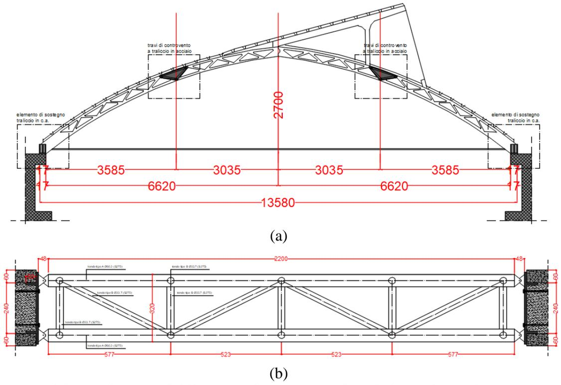
Fig. 12 – (a) Section of RC truss arch structures of roof; (b) steel truss beams as lateral force system in roof.
