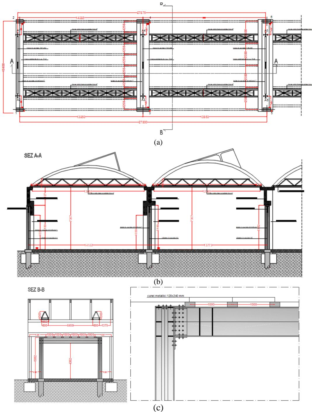
Fig. 11 – (a) View of plan with parallel RC frames and steel truss beams; (b) section and (c) details of steel frame.
