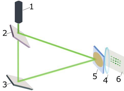
**Figure 2.** The experimental equipment for diffraction grating record: 1- Nd:YAG-laser, 2 – beamsplitter plate, 3 – mirror, 4 – lens, 5 – sample, 6 – screen
