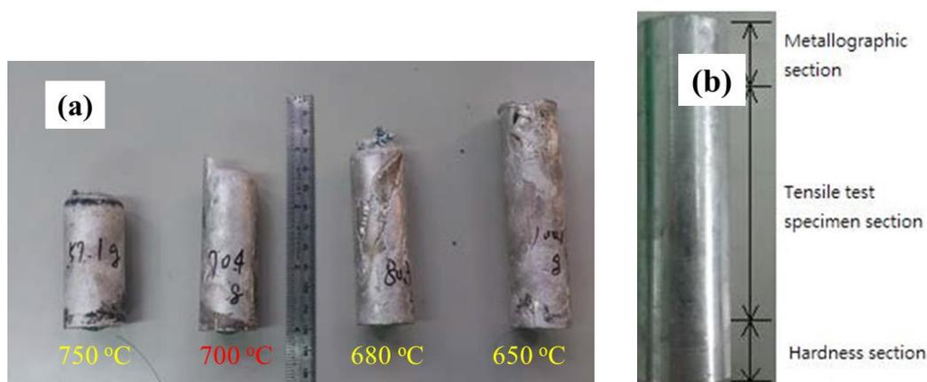
**Figure 2.** (a) Ingots of AZ31 at different temperature and (b) ingot sections for metallographic, tensile and hardness tests.
