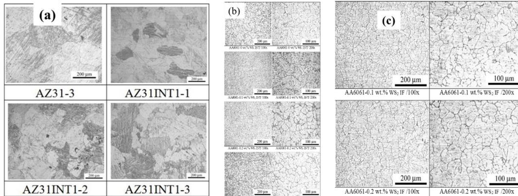
**Figure 6.** (a) Metallography of the pure Mg alloy and the different Mg alloys formulated with 1 wt% INT-WS<sub>2</sub>, (b) Metallography of AA6061 MMCs with added 0.1, 0.2 and 0.5 wt.% WS<sub>2</sub> INT and (c) Metallography of AA6061 MMCs with 0.1 and 0.2 wt.% WS<sub>2</sub> IF.
