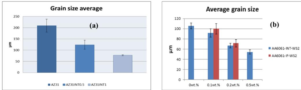
**Figure 7.** (a) Comparison between the grain sizes of the pristine AZ31 Mg alloy and the MMC's with 0.5 and 1 wt% of WS<sub>2</sub> nanotubes and (b) Grain size analysis of AA6061/ WS<sub>2</sub> INT MMCs and AA6061/ WS<sub>2</sub> IF MMCs.
