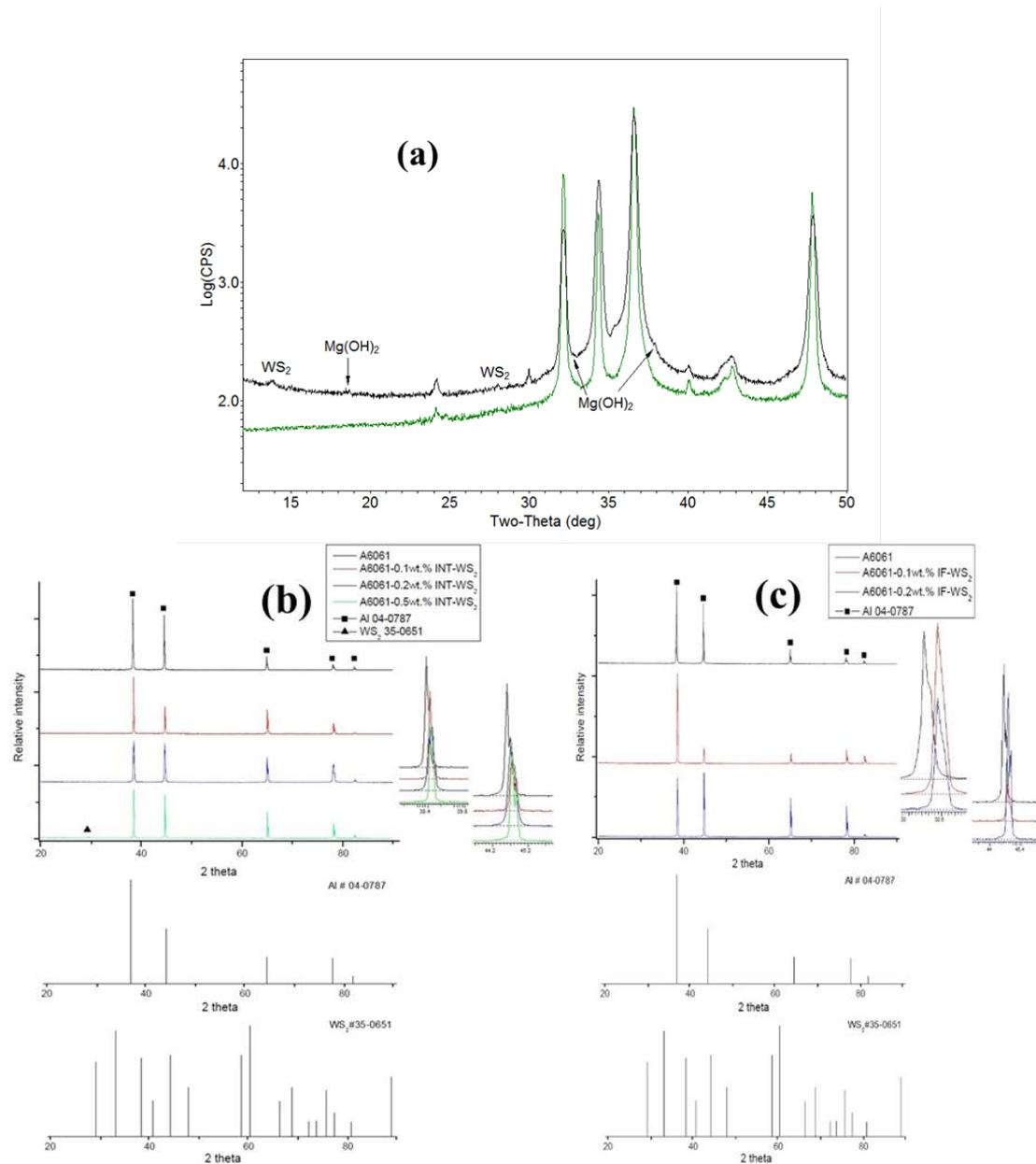
**Figure 3.** (a) XRD patterns of the AZ31INT0.5-1 sample and a pristine Mg alloy (green), (b) XRD patterns of AA6061/ WS<sub>2</sub> INT MMCs and (c) XRD patterns of AA6061/ WS<sub>2</sub> IF MMCs.
