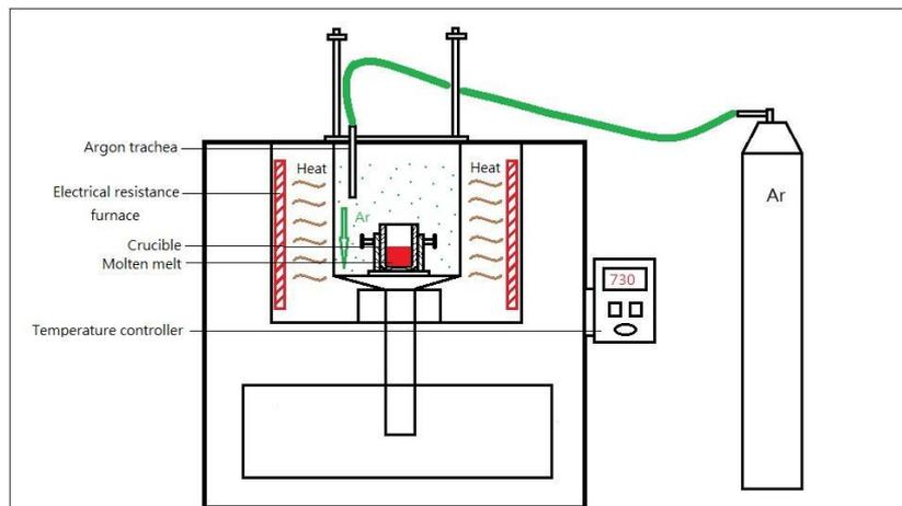
**Figure 1.** Schematic of stir casting furnace used for the fabrication of the Mg and Al MMCs.
