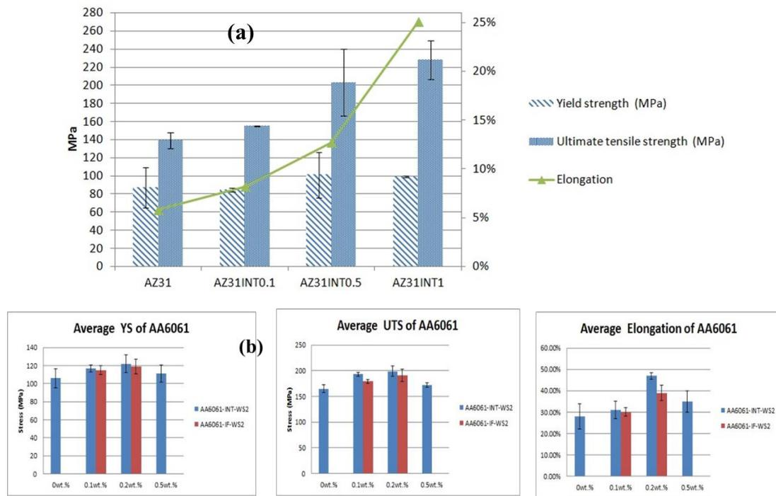
**Figure 5.** (a) Summary of the mechanical testing of the different Mg-alloy samples and (b) Summary of the mechanical testing of AA6061/ WS<sub>2</sub> INT MMCs and AA6061/ WS<sub>2</sub> IF MMCs.
