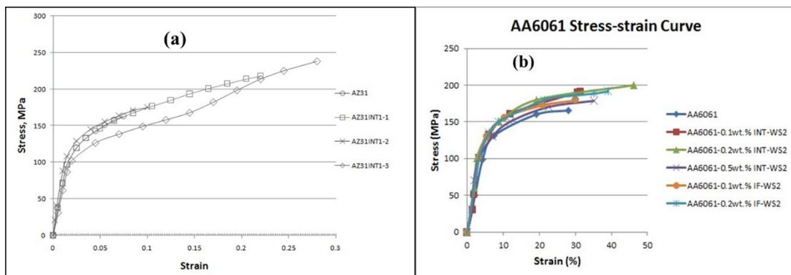
**Figure 4.** (a) Stress-strain curve (tensile test) of the pure Mg-ZA31 alloy and the Mg MMC with 1 wt% nanotubes (AZ31INT1-x; x=1-3) and (b) Stress-strain curve of AA6061/ WS<sub>2</sub> INT MMCs and AA6061/ WS<sub>2</sub> IF MMCs.
