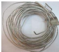
Fig. 1. A standard composition-pressed rod coil (granules of AD aluminum alloy and nanopowder).
