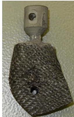
Figure 2. Sample for determining titanium rod-to-carbon composite bonding strength
