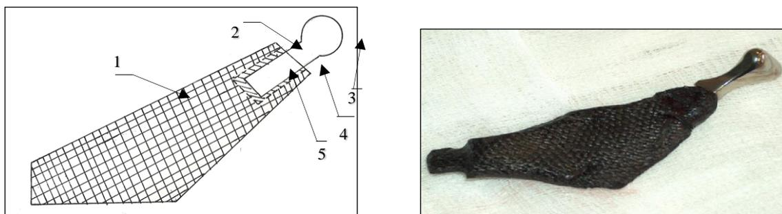
Figure 1. Implantation system used in repair of mandibular defects and prosthetic replacement of temporomandibular joint: a) structure schematic: mandibular part (1), articular part (2), head (3), neck (4), cylindrical connecting bar (5); b) finished structure
