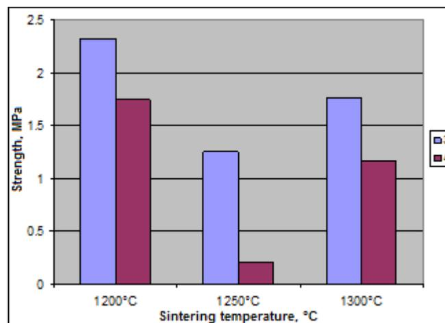
Figure 3. Titanium rod-to-carbon composite bonding strength as a function of the slip composition and the sintering temperature
