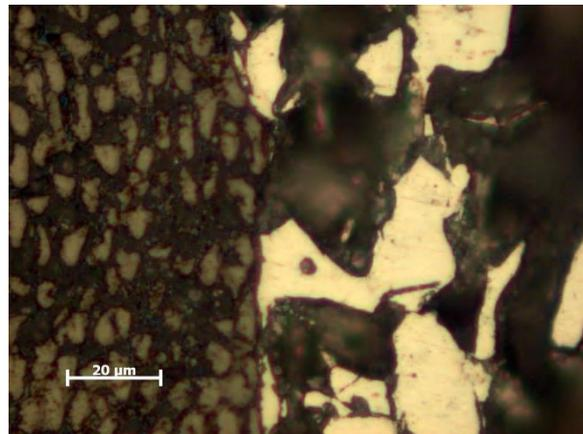
Figure 4. Microstructure of the carbon component and the titanium component after slip-aided sintering (sintering: 1200°C,  $\times 1000$ )
