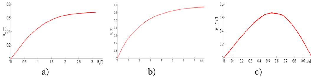
**Fig. 2.** Saturation curves for steel helix with quadratic cross-section, period  $d=10$  mm, and inner radius  $R_1 = 1$  mm. Dependences of undulator field  $B_u$  on: (a) axial field  $B_0$  ( $a=5$  mm,  $R_2 = 4.5$  mm), (b) helix thickness  $b$  ( $a=5$  mm,  $B_0 = 4$  T), and (c) helix axial size  $a$  ( $R_2 = 4.5$  mm,  $B_0 = 4$  T).
