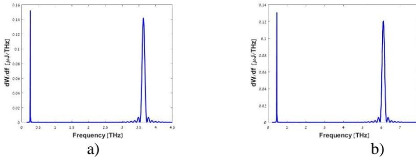
**Fig. 6.** Spectrum of radiation for a single point-like particle with charge 1 pC and energy 6 MeV passing 40 undulator periods in waveguide: a)  $d=10$  mm,  $D_w = 1.5$  mm and b)  $d=8$  mm,  $D_w = 1$  mm.
