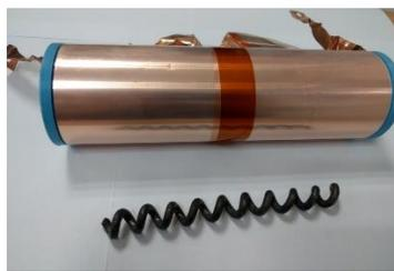
**Fig. 3.** Pulsed foil solenoid with strong magnetic field and helical insertion of 12-mm period used in measurements.
