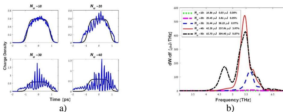
**Fig. 10.** Evolution of bunch density (a) and high-frequency parts of radiation spectra (b) for a bunch with charge 1 nC, radius 0.2 mm, duration 1.7 ps, and energy 6 MeV passing the distance of (16-64) cm in undulator with period of 8 mm and waveguide with diameter of 1 mm.
