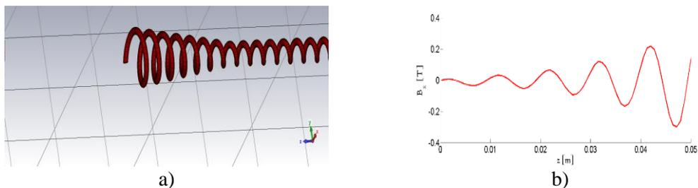
**Fig. 4.** Helical steel insertion with changing radius for adiabatic entrance of particles (a) and corresponding distribution of  $x$ -component of undulator field (b).
