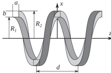
**Fig. 1.** Ferromagnetic helical insertion into solenoid.
