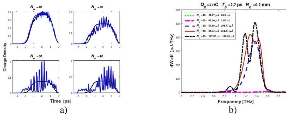
**Fig. 9.** Evolution of bunch density (a) and high-frequency parts of radiation spectra (b) for an extended bunch with charge 1 nC, radius 0.2 mm, duration 2.7 ps, and energy 6 MeV passing the distance of (10-40) cm in undulator with period of 10 mm and waveguide with diameter of 1.5 mm.
