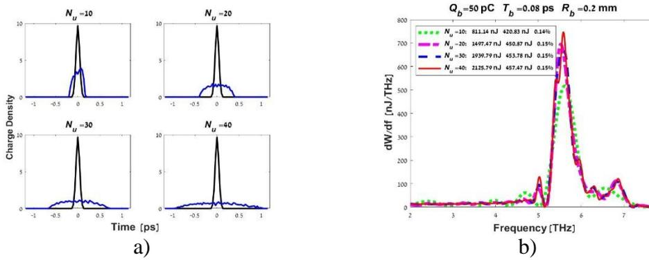
**Fig. 8.** Evolution of bunch density (a) and high-frequency parts of radiation spectra (b) for a bunch with charge 50 pC, radius 0.2 mm, duration 0.08 ps, and energy 6 MeV passing the distance of (10-40) cm in undulator with period of 8 mm and waveguide with diameter of 1 mm.
