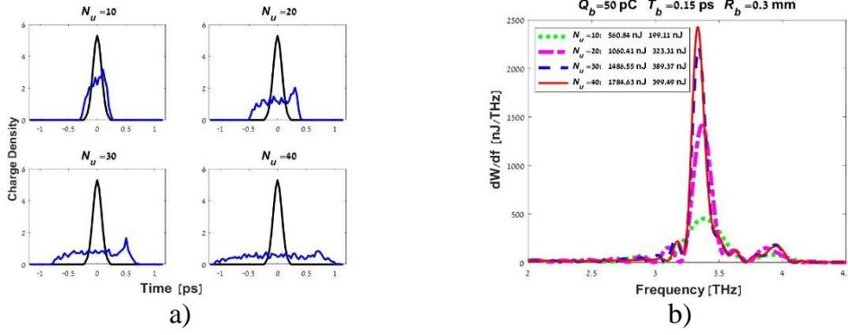
**Fig. 7.** Evolution of bunch density (a) and high-frequency parts of radiation spectra (b) for a bunch with charge 50 pC, radius 0.3 mm, duration 0.15 ps, and energy 6 MeV passing the distance of (10-40) cm in undulator with period of 10 mm and waveguide with diameter of 1.5 mm.
