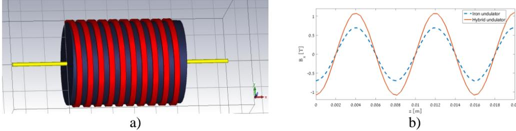
**Fig. 5.** A hybrid insertion consisting of a steel helix (“bolt”, red) placed inside a permanently magnetized helical block (“nut”, blue) with magnetization that is opposite to direction of the uniform field of a solenoid (a) and distributions of undulator field without and with a permanent block (b).
