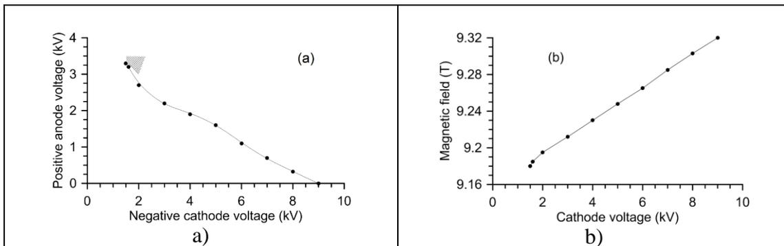
Fig. 6. Measured dependences of voltage on the first anode (a) and magnetic field (b) on the accelerating voltage in the regime of occurrence of gyrotron generation; shaded area corresponds to modulation of signal due to reflection of electrons.
