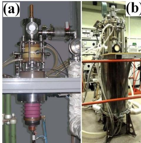
Fig. 4. LOGs with parameters 1 THz/80 kV (a) and 0.394 THz /30 kV (b).
