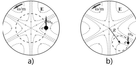
**Fig. 3.** The field of a  $TE_{mp}$  mode near the cavity axis coincides with the field of a rotating field  $2m$ -pole for an electron rotating around the cavity axis (a) or represents the set of all multipoles at the displaced electron rotation center (b); in the first case (LOG), radiation is possible only at  $m$ th harmonic, and in the second case (conventional gyrotron) it can be at any cyclotron harmonic.
