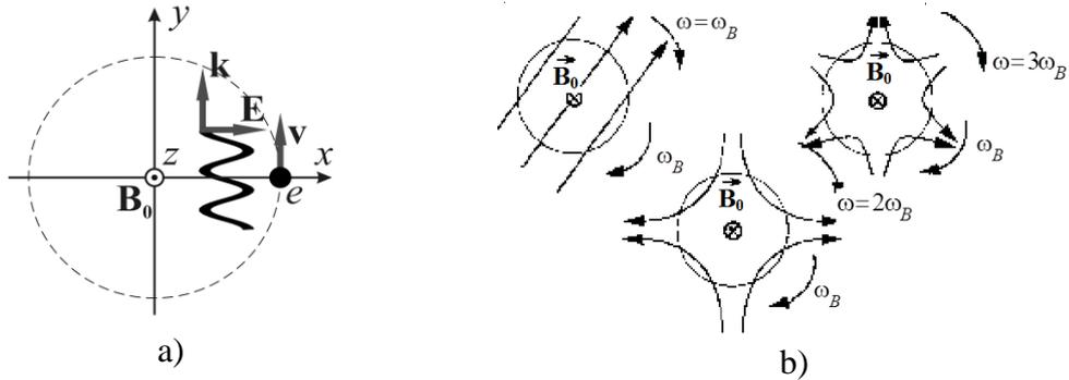
**Fig. 2.** The wave field on the trajectory of a particle that rotates with a cyclotron frequency (a) can be represented as a set of rotating field multipoles  $s = 1, 2, 3 \dots$  (b); one of co-rotating multi-poles can be in resonance with the wave.
