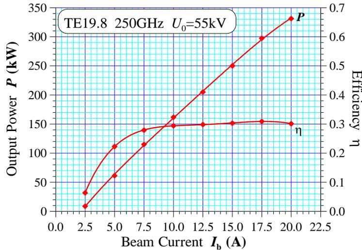
**Fig.4.** The output power and efficiency versus beam current observed at 0.25 THz gyrotron experiments [17].
