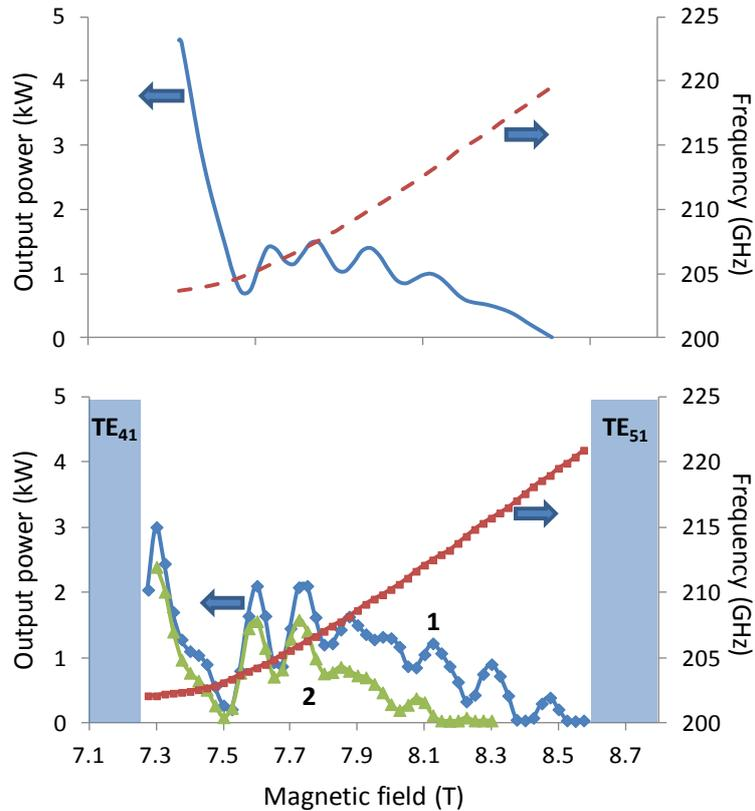
**Fig.5.** Gyrotron output power and radiation frequency vs. guiding magnetic field: the results of simulations based on self-consistent model for the cavity length reduced about three times in contrast with typical one (up) and the results of PIC simulations (down) for the same parameters and for two values of the relative transverse velocity spread, 20% (curve 1) and 50% (curve 2). The shaded area corresponds to the excitation of the parasitic modes [25].
