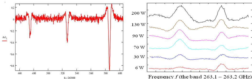
**Fig.7.** Examples of SO<sub>2</sub> spectrum for central frequency of about 0.5 THz and the spectrum lines measured with sensitivity of  $\sim 8 \times 10^{10} \text{ cm}^{-1}$  [29].
