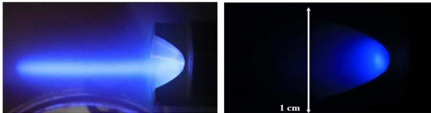
**Fig.6.** Gas discharge maintained at different initial gas pressure (left  $\sim 10^{-1}$  Torr, right  $\sim 10^{-2}$  Torr) by THz radiation. The signal from p-i-n diode corresponded to the power about 10 kW in a range 112-180 nm
