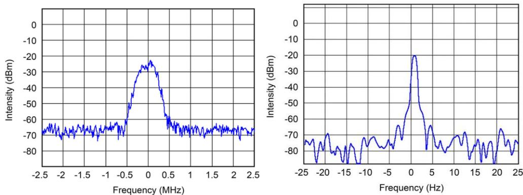
**Fig.3.** Experimental frequency spectrum of the free running gyrotron (left) and with phase-locked loop at an intermediate frequency with spans of 60 Hz (right) [16].
