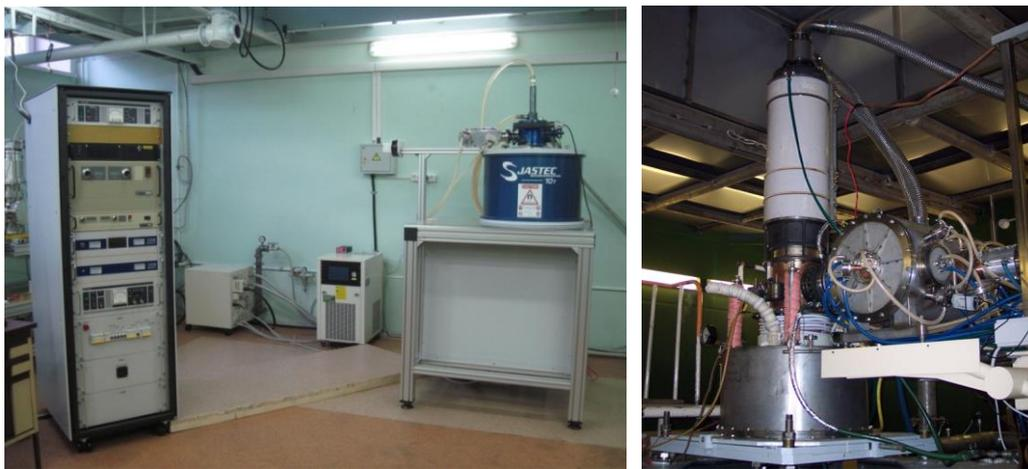
**Fig.2.** 0.26THz/1kW/CW system with a liquid helium free JM10T100 cryomagnet (JASTEC Ltd) at IAP RAS laboratory and 1 MW test facility in GYCOM experimental room.
