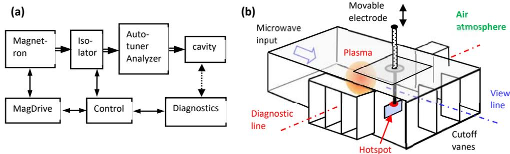
**Fig. 5:** A typical experimental setup for LMH-plasma generation [32]: (a) A block diagram of the experimental instrumentation, and (b) the microwave cavity.
