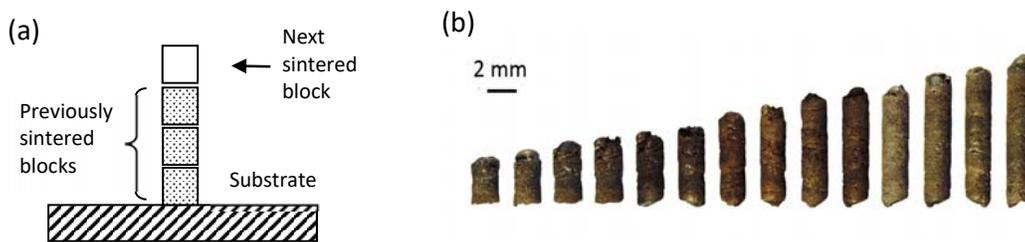
**Fig. 8:** Additive manufacturing (3D printing) of metal powders by LMH [36]: (a) A conceptual scheme of the stepwise LMH-AM process. (b) A 2-mm $\varnothing$  rod constructed in 14 consequent steps from bronze-based powder.
