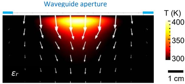
**Fig. 3:** A numerical simulation of a hotspot evolved in an arbitrary material placed in front of a waveguide aperture ( $\epsilon_r = 2.0 - j0.1(T - 290)$  and WR340, respectively) [6]. The LMH effect is evident by the temperature profile, as well as the focusing-like convergence of the Poynting vector (denoted by the white arrows).
