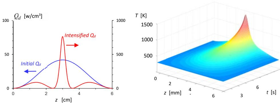
**Fig. 2:** A numerical example of LMH in a 1-D cavity [7]. (a) Initial and final profiles of the dissipated power density  $Q_d$  along the cavity, from the fundamental-mode excitation to the LMH instability and hotspot. (b) The localized temperature profile along the cavity, and the hotspot evolved.
