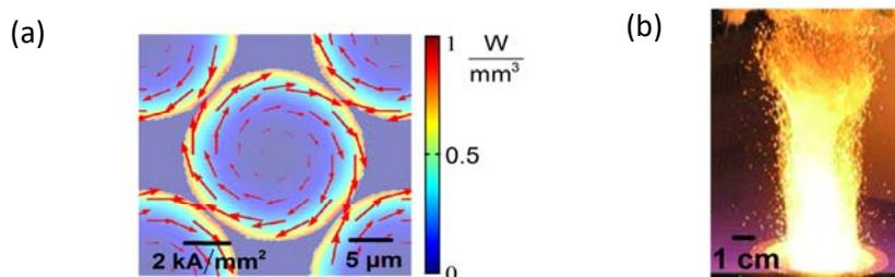
**Fig. 7:** LMH of metallic powders. (a) Eddy currents induced in copper powder [41]. (b) A thermite flame ignited by LMH intensification [37].
