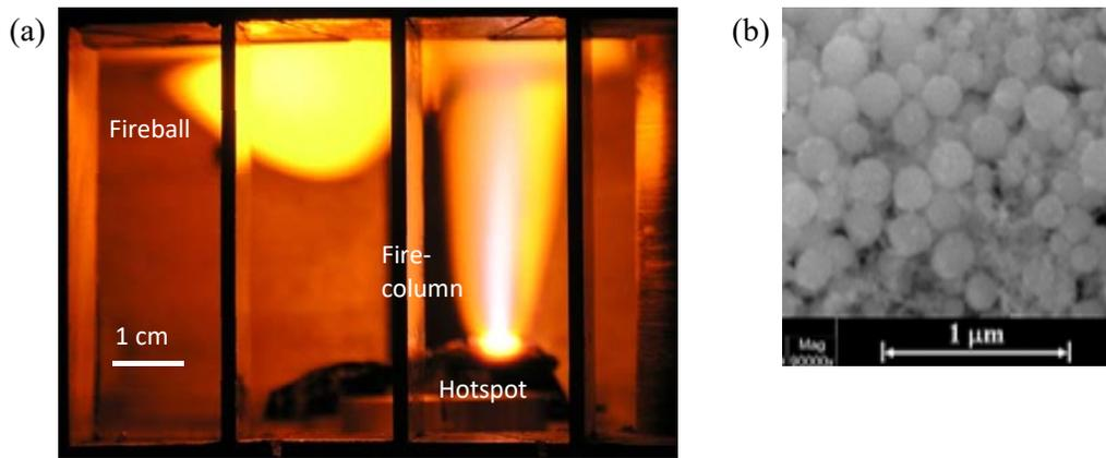
**Fig. 6:** Plasmoids ejected by LMH from a hotspot in glass [31]. (a) The hotspot in the solid substrate, the fire-column ejected, and the secondary fireball evolved (captured together). (b) Nano-particles produced by LMH generated dusty plasma, as observed by SEM.
