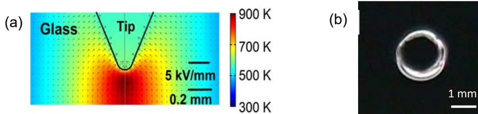
**Fig. 4:** LMH effect in glass irradiated by a coaxial open-end applicator using an LDMOS-based microwave-drill [17]: (a) The simulated spatial temperature and electric-field distributions at the hotspot, and (b) an image of a ~1.6-mm $\varnothing$  hole made by LMH in glass.
