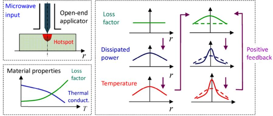
**Fig. 1:** The induced thermal-runaway instability and the self-focusing effect [5].
