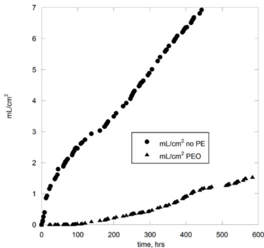
Figure 7. Plots of the gas evolution rate for the oxidized and not oxidized samples of MRI230D alloy.
