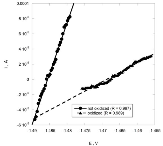
Figure 6. LPR plots for the PEO oxidized and not oxidized samples of MRI230D alloy.
