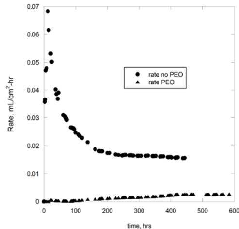
Figure 8. The time dependencies of the gas evolution rates for the oxidized and not oxidized samples of MRI230D alloy.
