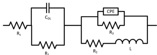
Figure 4. An equivalent circuit best fit to the measured EIS spectra.
