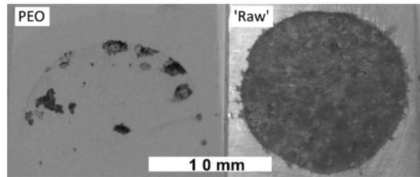
Figure 2. The surfaces of a 'raw' not oxidized sample (right) and of a PEO treated sample (left) after some days of immersion into 3% NaCl. Only the round window was open for the corrosion process, the rest of the surface sealed by a polymer.
