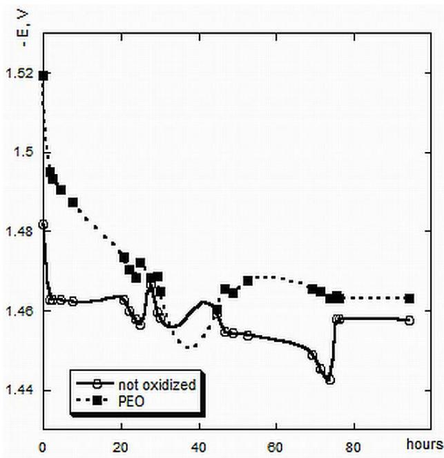
Figure 1. Stabilization of the corrosion potential (vs. Ag/AgCl) of MRI230D in 3% NaCl.
