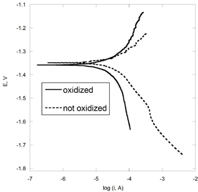
Figure 5. Tafel polarization plots for the PEO oxidized and not oxidized samples of MRI230D alloy.
