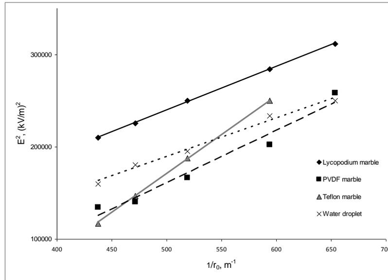
FIG. 4. Squared critical electric field versus inverse radius,  $1/r_0$ , of the spherical marble of an equivalent volume. Different slopes resemble different surface energies at the marble/oil interfaces.
