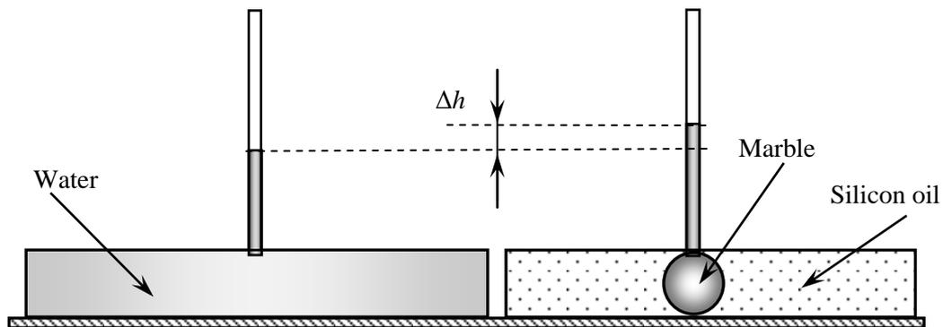
FIG. 5. Scheme of the measurement of surface tension with capillary method.
