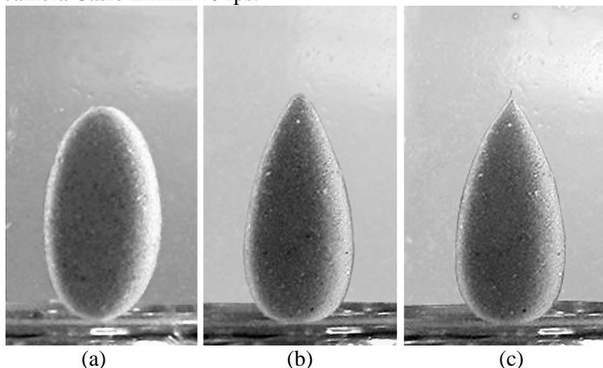
FIG. 2. Lycopodium-coated marble deformed in the electrostatic field of  $0.48 \cdot 10^6$  V/m to the prolate-spheroid shape (a). The Taylor cone formation at the end of marble (b) followed by jetting (c) at the field value  $0.51 \cdot 10^6$  V/m. Volume of the marble was  $20 \mu\text{l}$ .
