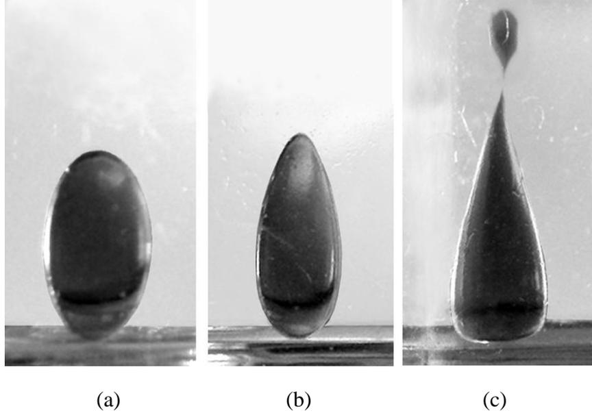
FIG. 3. Water droplet deformed in the electrostatic field of  $0.41 \cdot 10^6$  V/m to the prolate-spheroid shape (a). The Taylor cone formation (b) followed by jetting (c) at the field value of  $0.42 \cdot 10^6$  V/m. Volume of the droplet was  $20 \mu\text{l}$ .
