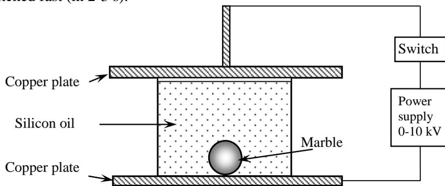
FIG. 1. Scheme of the experimental unit used for electrostatic actuation of marbles.
