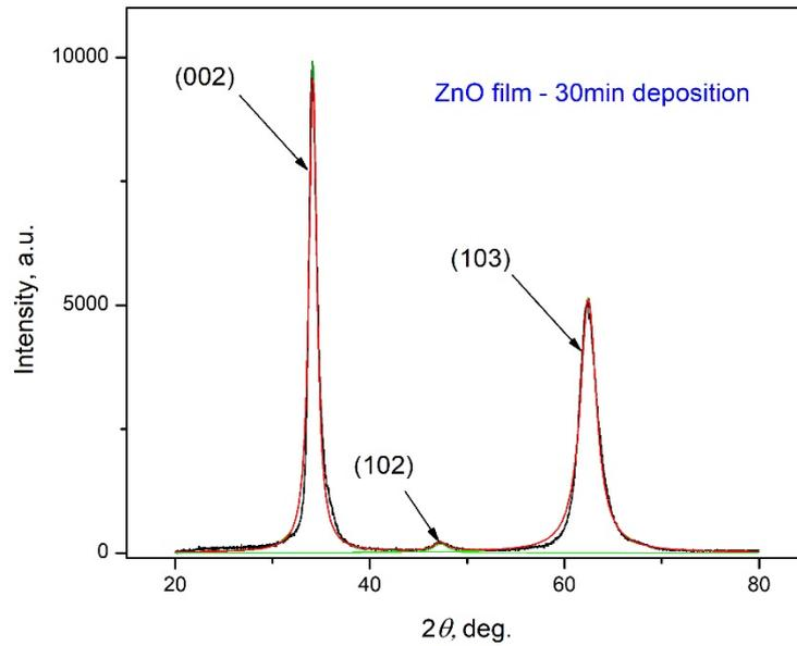
Fig. 1. XRD profile of ZnO film with 30 min sputtering duration.
