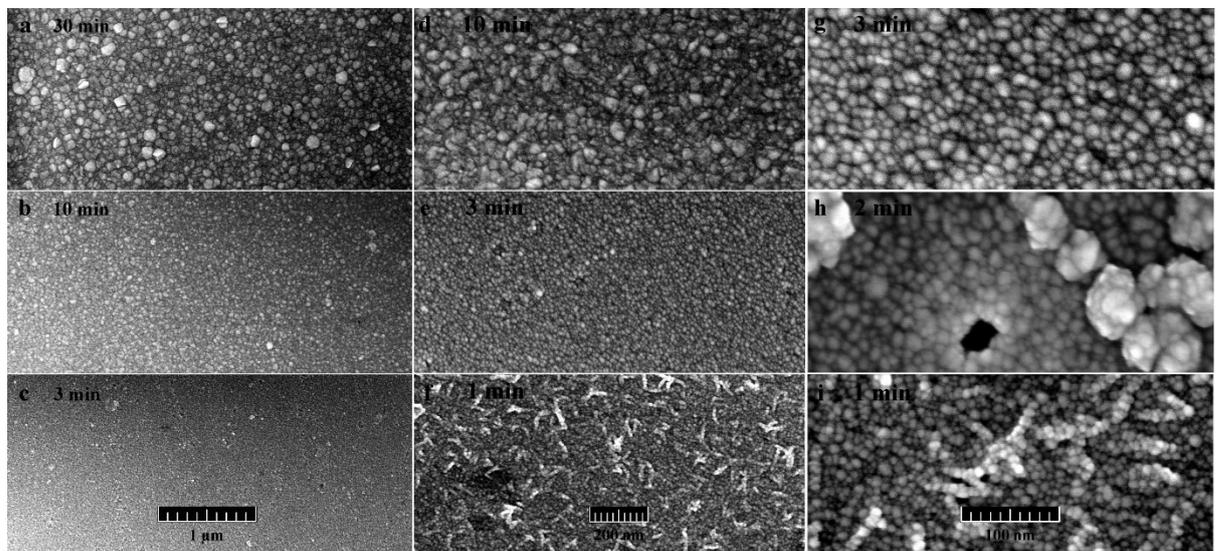
Fig. 2. SEM images of ZnO films with different deposition times.
