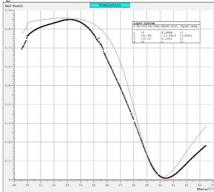
Fig. 5. The processing of SPR curve for ZnO film deposited on a glass substrate for 60 s.
