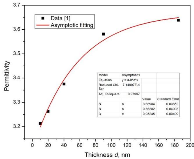
Fig. 4. Thickness dependence of permittivity for nanoscale ZnO films.
