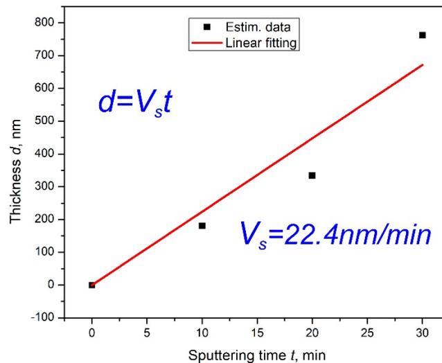
Fig. 3. The deposition rate and the thickness of ZnO films estimated with PW method.
